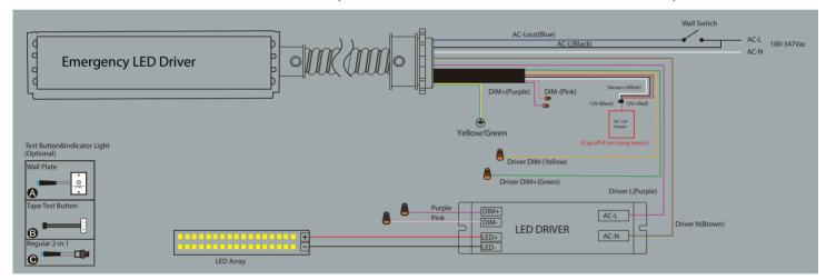
CAUTION: The Emergency LED driver must connect to 0-10V dimming wires(DIM+,DIM-) of the luminaire if the LED luminaire power is exceed the emergency LED driver power.
