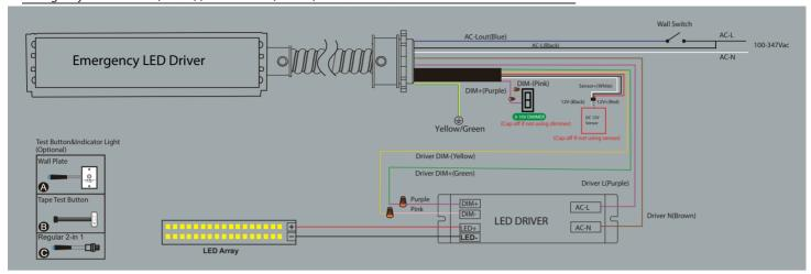
2. For LED luminaires with non 0-10V dimmable LED driver (\* LED DRIVER INPUT POWER ≤ EMERGENCY OUTPUT POWER)
