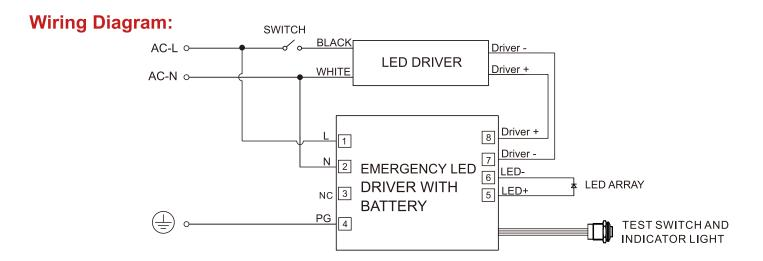
1.DO NOT MATE CONNECTOR UNTIL INSTALLATION IS COMPLETE AND AC POWER IS SUPPLIED. 2.TEST ACCESSORY LEADS-OBSERVE PROPER POLARITY WIRING.
