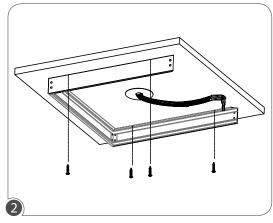
Assemble and install 3 sides of SMK frame on the ceiling. Make sure the wires are long enough for step 3.
