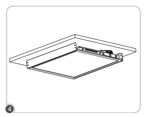
Check to see if the fixture sit properly on the inner flanges of the SMK frame.
