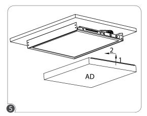
Slide in the **AD** part (Acrylic Drop) underneath the fixture through the SMK frame.
