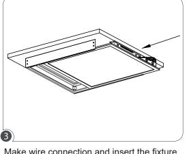
Make wire connection and insert the fixture to the frame all the way.
