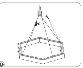
Cut the extra cable in the center once finish adjusting the suspension length.
