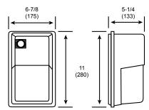
Specifications: MWP1 Height: 11 (280) Width: 6-7/8 (175)
